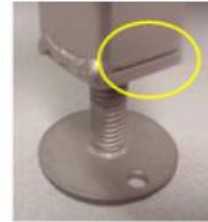
Fig. 20. Hollow square tubing not hermetically sealed (missed weld on one side of the leg)
